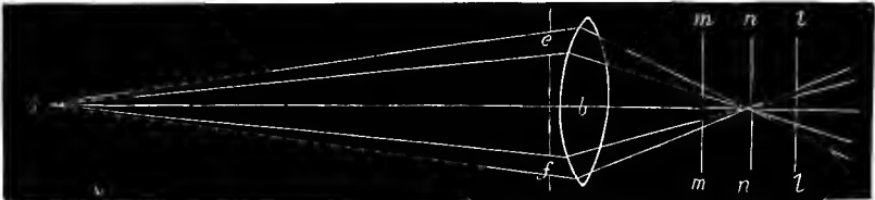
Fig. 350.—Scheiner's Experiment—an experiment to determine the minimum distance of distinct vision.
